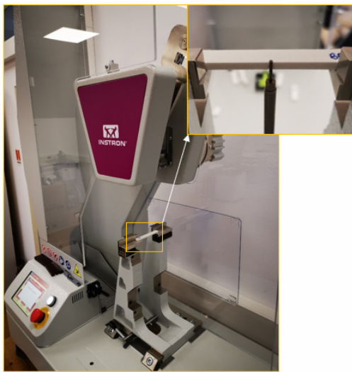
Fig. 2. Specimen on Instron CEAST 9050 instrumented impact testing equipment.
